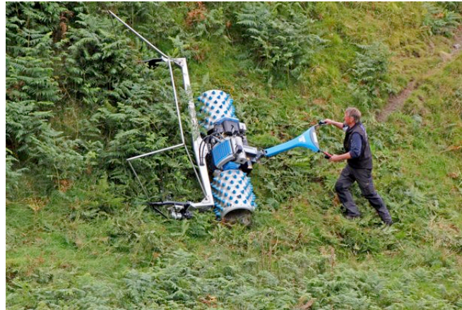
Brielmaier cutters, demonstrated in Cumbria in 2015, can tackle steep slopes. The cutters can cost £20-30,000 and some of the machines can also mulch. Other machines are needed to rake the material where it can be baled. Photo credit: Roland Priebe.
